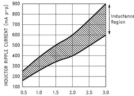
**Figure 18. Peak-to-Peak Inductor Ripple Current vs Load Current**
