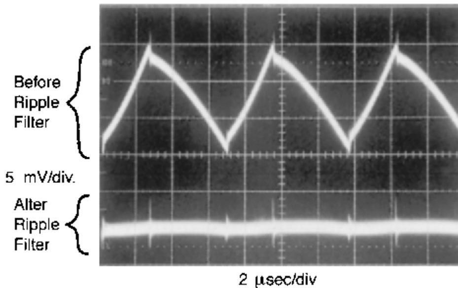
**Figure 17. Post Ripple Filter Waveform**
