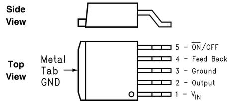
**Figure 2. Surface Mount Package 5-Lead TO-263 (S)**
