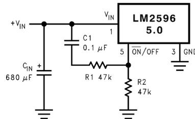
**Figure 21. Delayed Startup**
